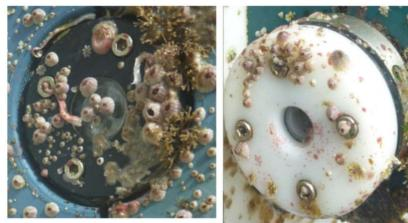
Fig. 18. Antifouling system applied to optical sensor submerged in natural seawater for 4 months in France. Left – unprotected; Right - protected
