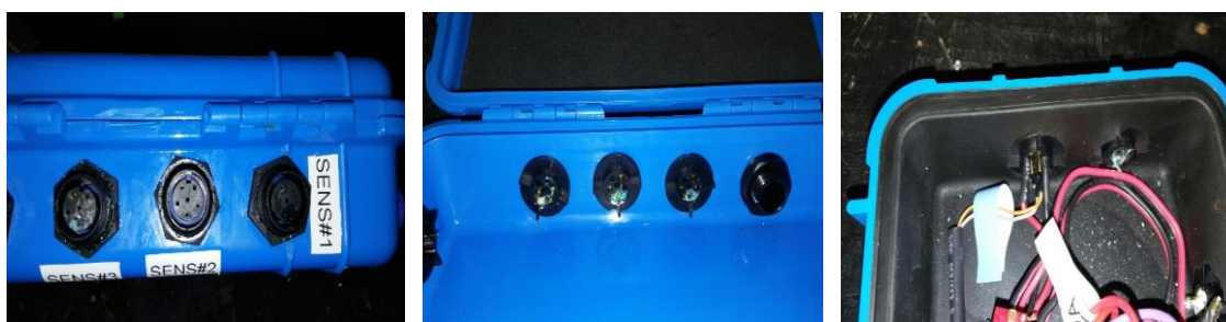
Figure 7. Result of water filtering inside Sensor Integration Box.
